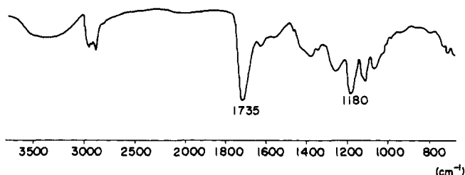
Figure 1. Ir spectrum of polymer 2a from 2-hydroxyethyl acrylate (1a).
